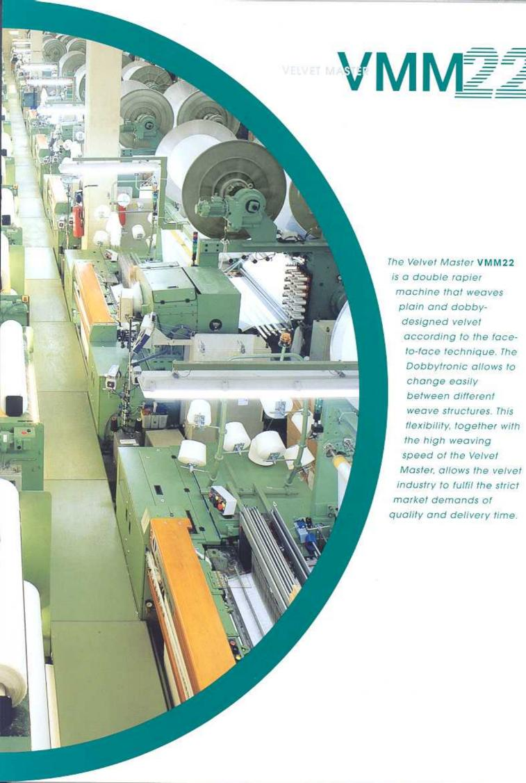
The Velvet Master VMM22 is a double rapier machine that weaves plain and dobbydesigned velvet according to the faceto-face technique. The Dobbytronic allows to change easily between different weave structures. This flexibility, together with the high weaving speed of the Velvet Master, allows the velvet industry to fulfil the strict market demands of quality and delivery time.
