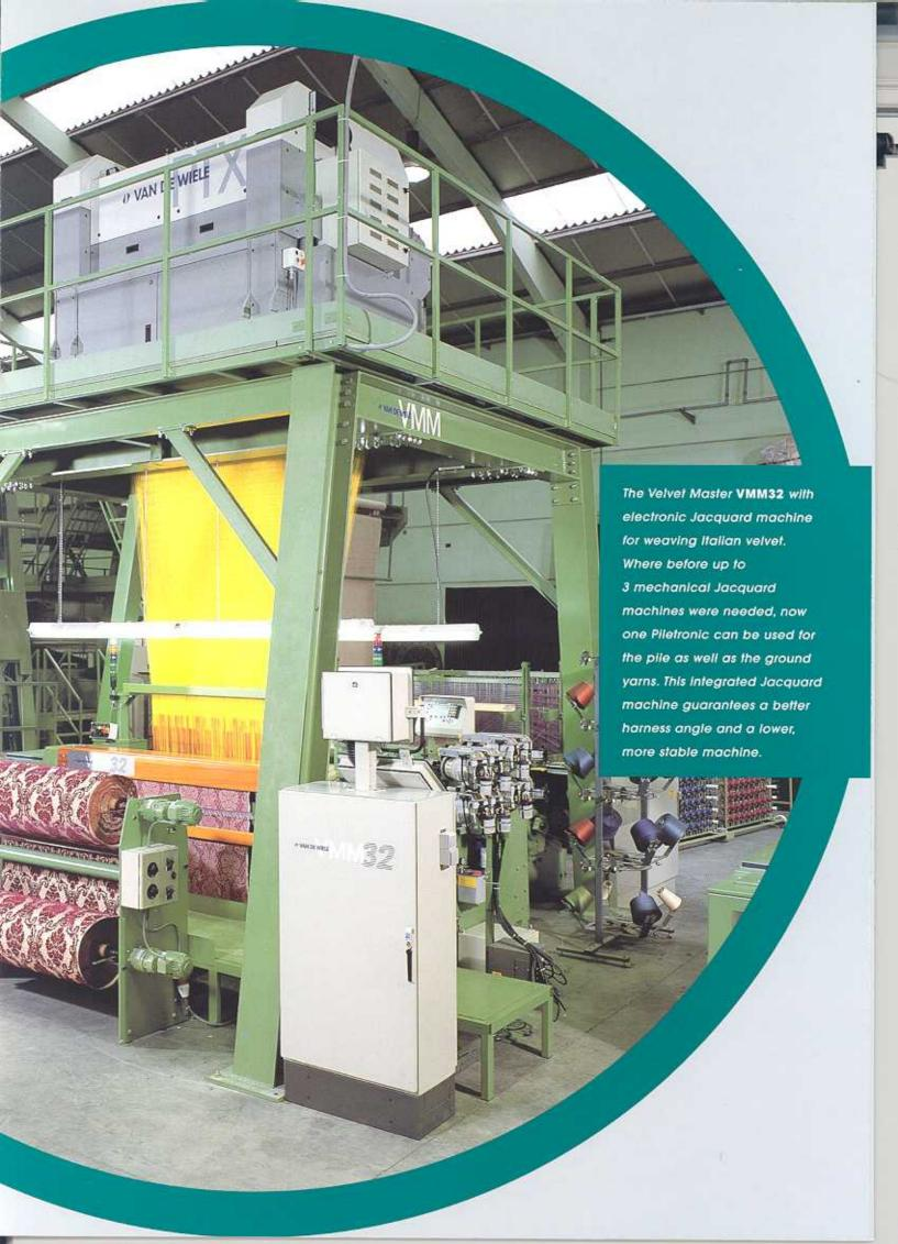
Because of the menustructured microprocessor and the extended operation panel, the machine is easy to control. The fillings run from the prewinders through a filling brake and an electronic stop motion to the filling scissors.
