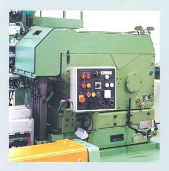
The Dobbytronic DTR allows to weave a number of new weave structures. Besides the already known, new weave structures with 10 pile, 6 ground and 4 edge frames or 8 pile, 8 ground and 4 edge frames can be woven. The Dobbytronic is programmed by a user friendly microprocessor. This gives an extended number of functions like setting the machine parameters, production follow up,...
