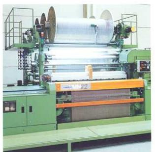
The Velvet Master VMM22 is equipped with a pile beam stand with direct electronic let-off.
