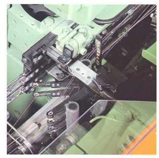
The pneumatic filling selector allows to choose between 2x4 colours. This gives additional ground effects when weaving Italian velvet. The new filling scissors can handle a broad range of different fillings.
